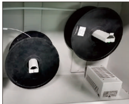
Filament dry room have 2 temperature options to set. (45 degree /65 degree.) Note: The PLA,PVA,HIP filaments are disable the drying function of the consumables bin.
