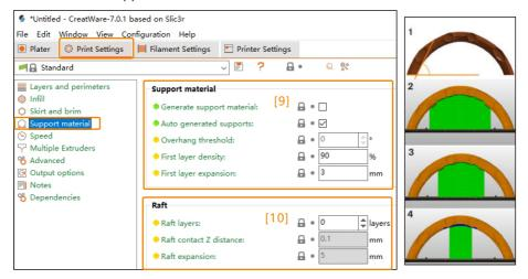
7.5.2 Raft[10]:Creates a raft below the part that can help with adhesion and provide a clean level surface to begin the print.
