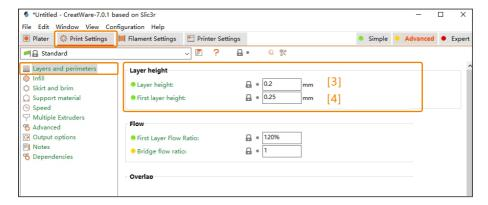
7.2.2 First layer height[4]: It refers to the height of the first layer of printing, generally greater than 0.2mm. This parameter can compensate the errors of the platform and make the model stick to the platform better.
