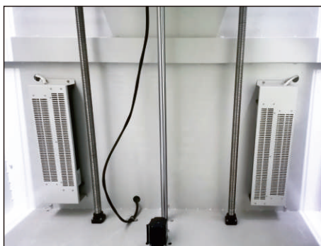
Hot Chamber system can make inside temperature up to 60 degree.
