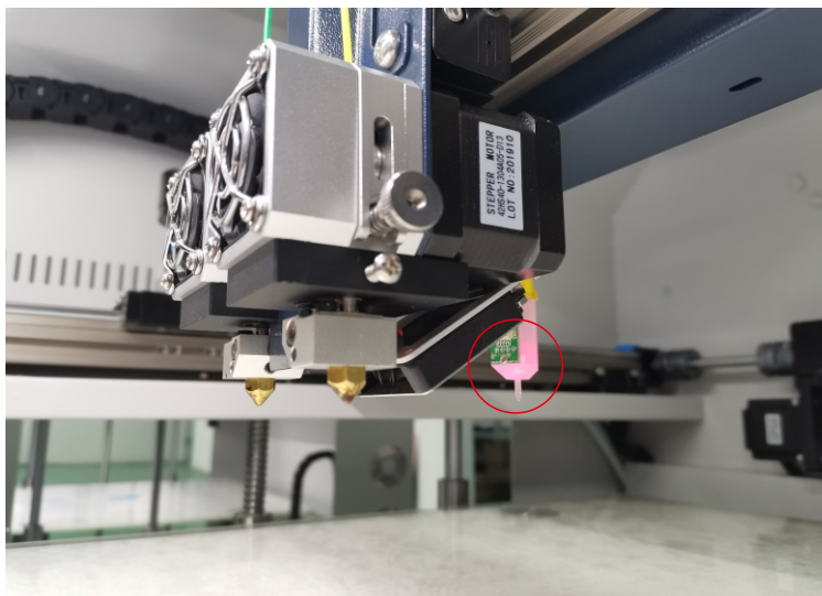
Auto leveling system (Available on D600 Pro) Auto-leveling working plate make leveling easily
